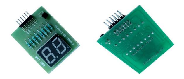
This module is based on a simple principle of switching digit enable signal. Digit enable signal is switched by a simple inverter which is made of a NPN transistor and resistor. The PCB blueprint shown below for reference to the users.
